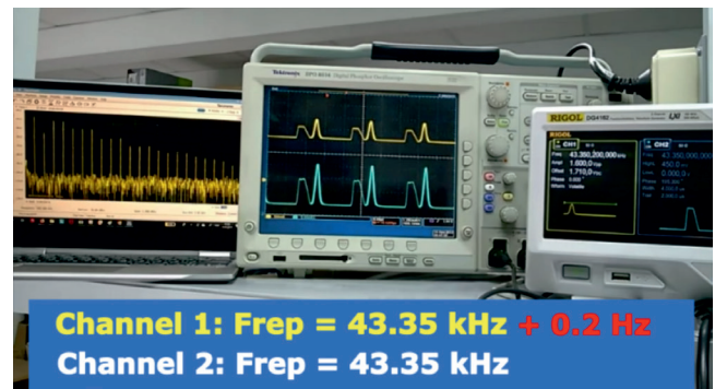
Figure 4. Captured video of on-the-lasing continuous modification of the laser pulse pattern structure. The instrumentation displayed left-to-right: an RF spectrum analyzer measuring the RF spectrum of the laser pulse pattern train, a digital oscilloscope measuring the modulation pulse pattern train (upper oscillogram) and the corresponding laser pulse pattern train (lower oscillogram), and a dual-channel RF AWG forming the modulation pulse pattern train. The inset indicates the repetition frequencies set for each AWG channel.
