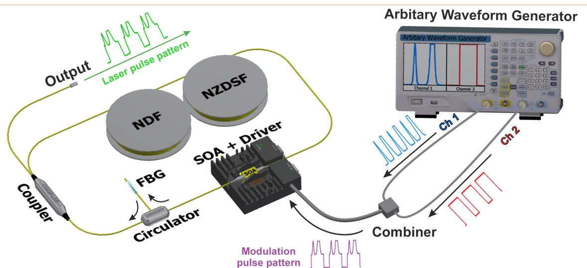
**Fig. 1** Mode-locked gain-modulated\* SOA-fibre laser implemented for generation of arbitrary laser pulse patterns and waveforms.
