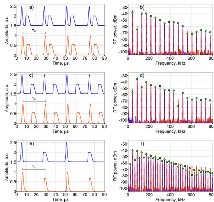
**Fig. 2** Oscillograms (a, c, e) and corresponding RF spectra (b, d, f) measured for modulation patterns (blue) and for laser pulse patterns (red). Green circles indicate theoretical spectra of desirable patterns.
