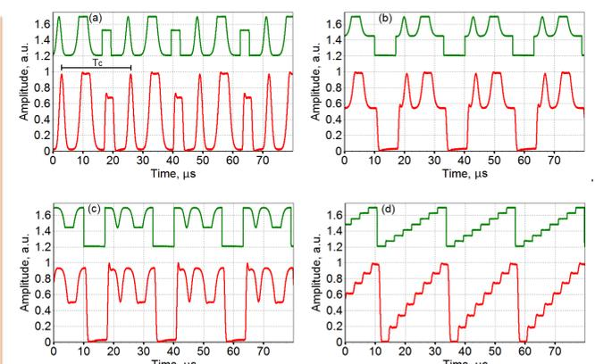
**Fig. 3** Oscillograms of complicated forms of driving electrical signal (green curves) and resulting laser pulse patterns/waveforms (red curves).
