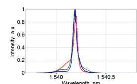
**Fig. 4** Optical spectra of generated laser waveforms: blue curve corresponds to the waveforms of Fig. 3(b), green curve to Fig. 3(c), red curve to Fig. 3(d).
