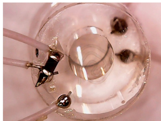
Fig. 9. Photographs of the cell windows with deposited conductive heating elements.
