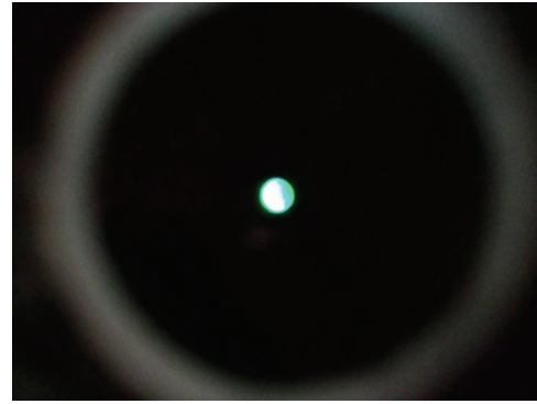
Figure 10. Photograph of the TH beam ( \lambda/3 = 520 \text{ nm} ) for generation in a 550-nm-thick RR-P3HT film on a substrate and pumping from the polymer side by near-IR radiation ( \lambda = 1560 \text{ nm} ), fed to the sample through a fibre.
