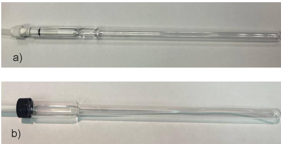
Figure 8. NMR tubes a) standard 10 mm in diameter tube b) tube with PTFE capillary
