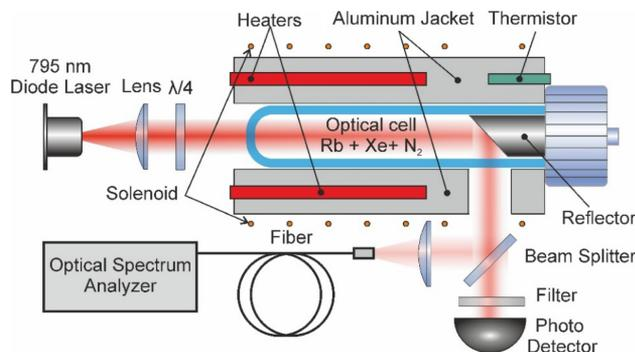
**Fig. 1.** Schematic diagram of the experimental prototype of a tabletop xenon hyperpolarizer.
