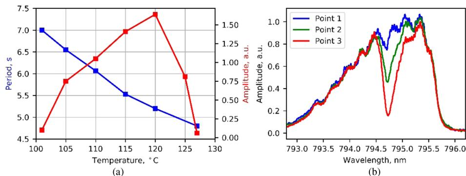
**Fig. 3.** (a) Dependence of oscillation period (blue curve) and amplitude (red curve) from temperature; and (b) The spectrum of radiation transmitted through the optical cell at the moments of the highest (blue curve), middle (green curve) and lowest (red curve) transmittance (points P1, P2, P3 in Fig. 2(c), respectively). A dip at the wavelength of 794.7 nm corresponds to the D1 absorption line in rubidium.
