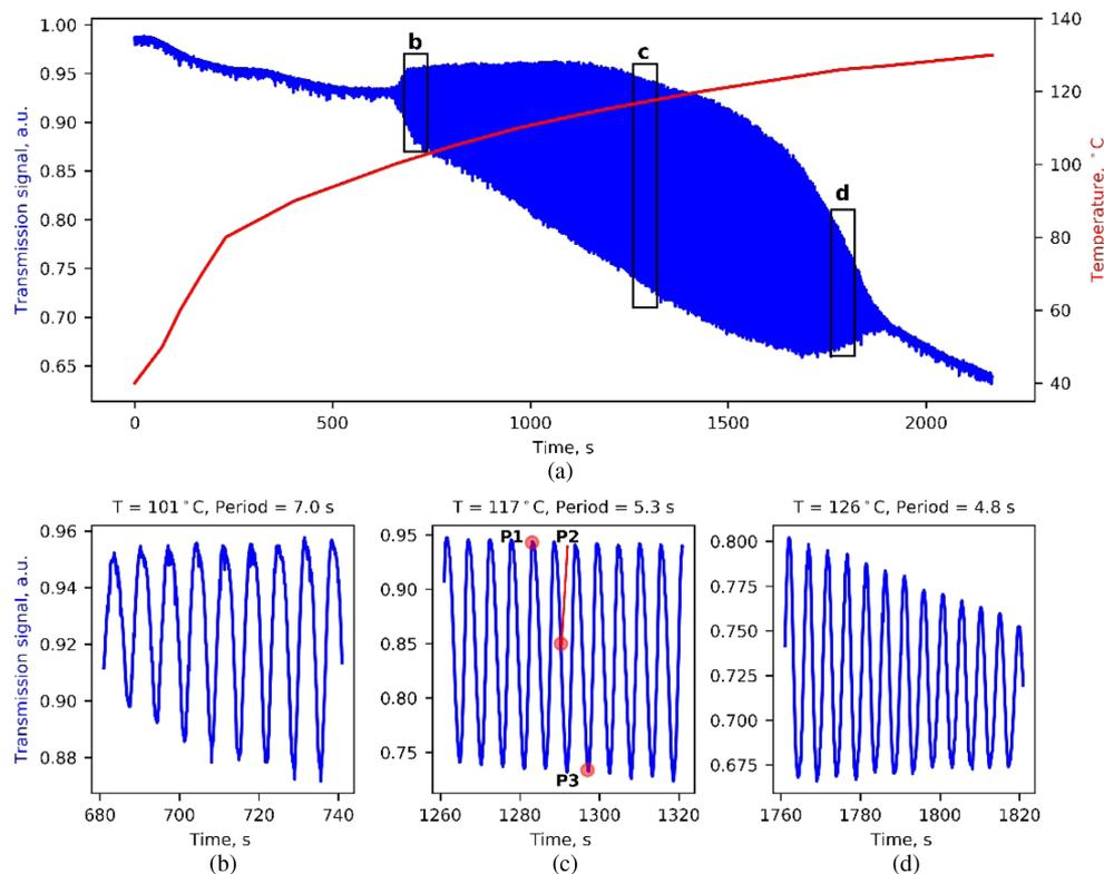
**Fig. 2.** Time trace of the radiation power transmitted through the Rb cell during the process of heating. Partial pressures are 150 kPa for xenon and 250 kPa for nitrogen, P1, P2, and P3, markers correspond to the time points at which the transmitted radiation spectra presented in Fig. 3(a).
