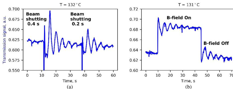
**Fig. 4.** Excitation of transient damped oscillations of the transmitted radiation intensity at the temperature beyond the domain where continuous oscillations occur by: (a) shutting the beam off for various amounts of time; and (b) by switching the longitudinal magnetic field on and then off.
