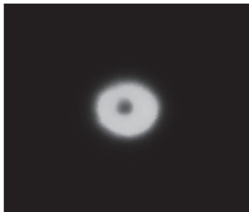
Figure 8. Spot of unabsorbed pump radiation, observed with the aid of a luminescence IR visualiser at the converter output.
